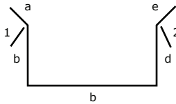
Box Gutter with Double Upturns
