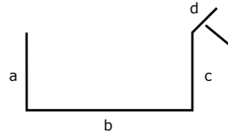
Box Gutter with Single Upturns
